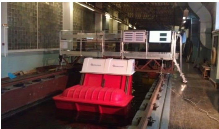
Figure 1 – The wave converter prototype made at the scale of 1:2.5 installed on a special testing rig in the ripple tank of the Krylov Research Center in order to verify the operation and to improve individual structural elements
