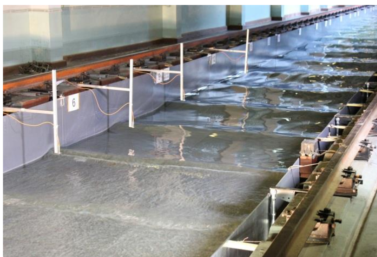
Figure 2 - Model of the Golubaya Bay seabed in the Krylov Research Center ripple tank and the wave performance in shallow water near the water edge
