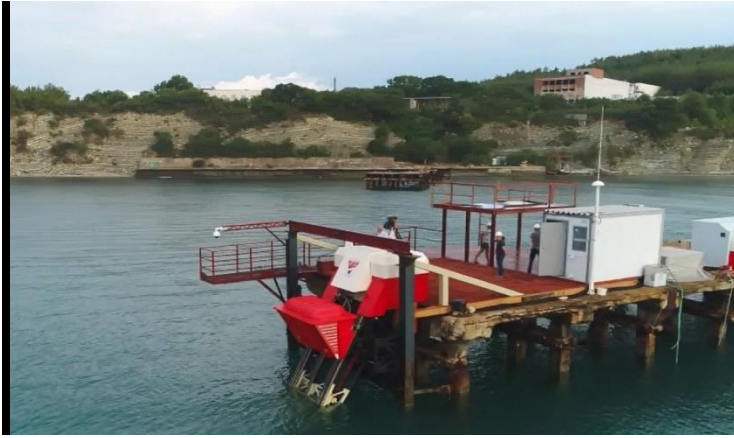
Figure 7 - The wave converter prototype made at the scale of 1:2 and installed in the Golubaya Bay of Gelendzhik (the Black Sea Coast)
